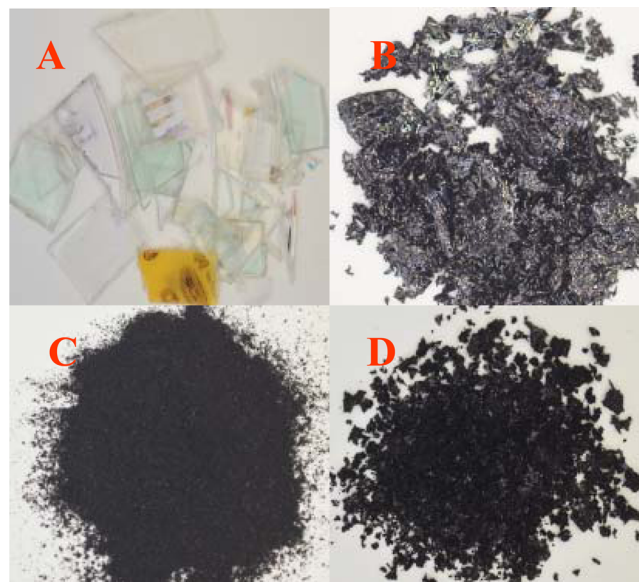
Figure 1. Photographs of disc fragments (A), C carbon (B), and C-KOH-4 (C), and C-CO 2 -8 (D) activated carbons.
